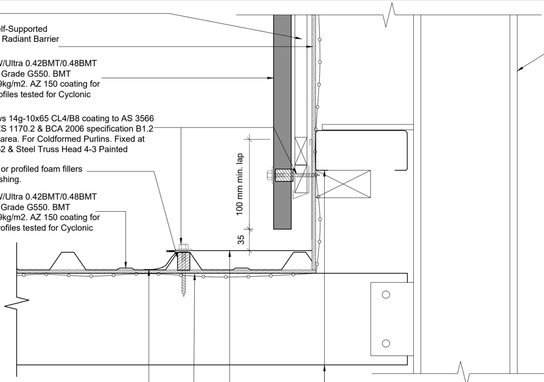
Flashguard Soft Edge flashing for metal roof accessories
